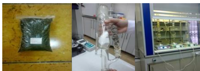
Figure 2 – Extraction of soil samples in the Soxhlet apparatus
